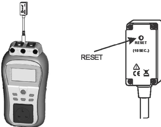
It is recommended to reset the instrument's A1436 BT dongle before proceeding with further steps. A1436 BT dongle can be reset by holding the Reset for at least 10 seconds as shown on the right picture.
