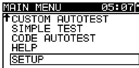
4. Enter SETUP menu using TEST button and move down to COMMUNICATION.
