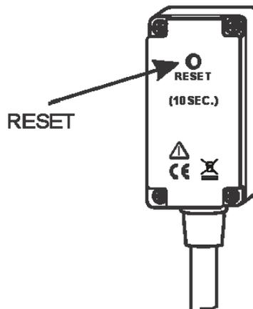
It is recommended to reset the printer`s A1436 BT dongle before proceeding with further steps. A1436 BT dongle can be reset by holding the Reset for at least 10 seconds as shown on the right picture.
